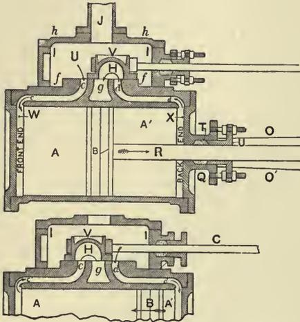
Figs. 20 (above) and 21.—Sections of a Locomotive Cylinder.
