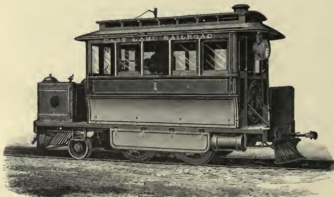
Fig. 13.—Locomotive for Street Railway. By the Baldwin Locomotive Works.
