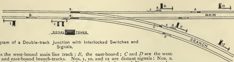
Diagram of a Double-track Junction with Interlocked Switches and Signals.
