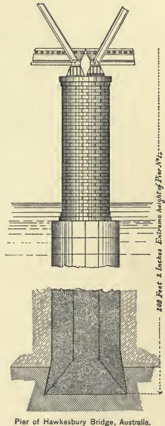
method of sinking these great foundations. The removal of material must be made with such systematic regularity that the structure shall descend evenly and always maintain its upright position.
