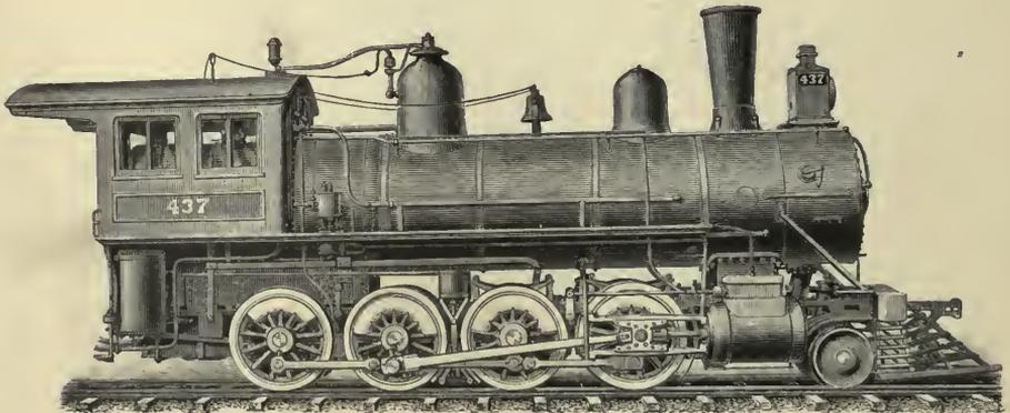
Fig. 30.—Consolidation Locomotive. By the Pennsylvania Railroad Company.
