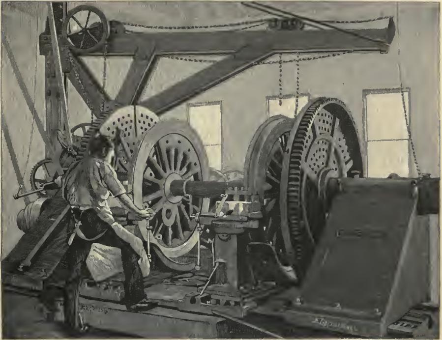
Fig. 25.—Turning Locomotive Tires.
